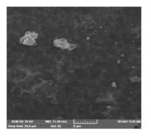
Scanning electron microscope image of Silver synthesised by Curculigo orchioides extract. The image clearly indicates the particle size range of our nanoparticles to be within 84.5 nm.
