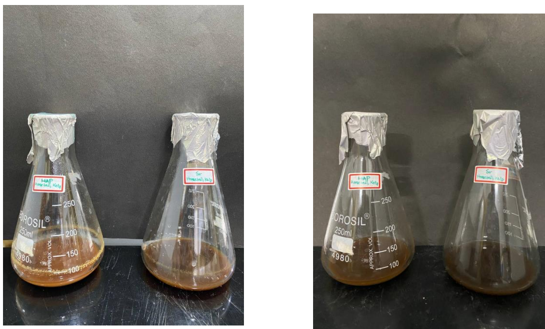
Figure 1: Visual observation showing the colour change from pale brown to dark brown indicating the formation of strontium and hydroxyapatite nanoparticles
