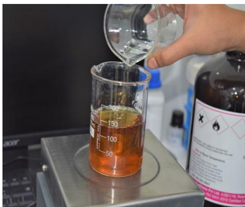
Fig 2: Represents the weighing of magnesium chloride salt which was further stirred by magnetic stirrer
