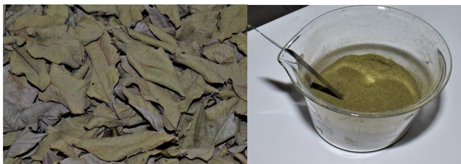
Fig 1: Represents the guava leaves that were dried for 2 week and grinded to form a fine powder
