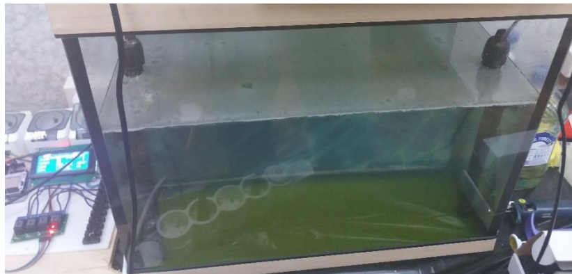
Fig.9: The surface of the suspension is covered with a thick organic film, 2-3 mm thick, a sapropel 2 mm thick has formed at the bottom of the aquarium, including dead Chlorella cells
