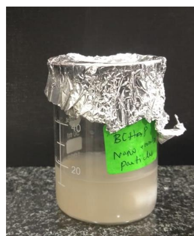
1a. 0.010 g of black cumin hydroxyapatite powder 1b. Mixed in 10mL of distilled water 1c. Thymoquinone mixture
