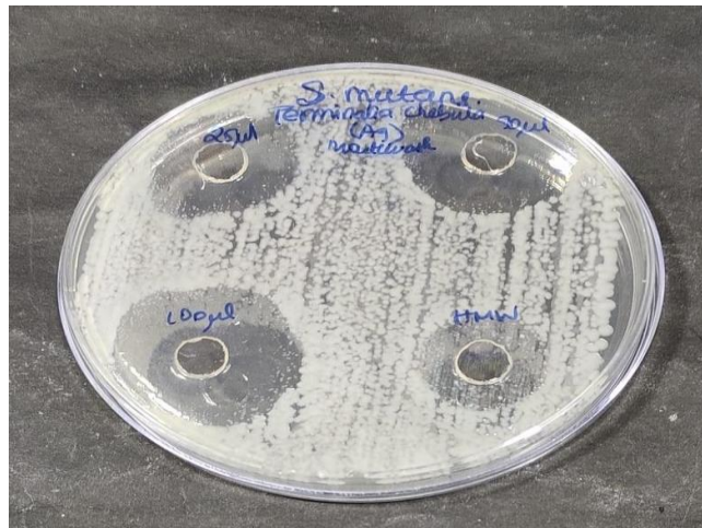
Fig.5: Showcasing the effect of various concentrations of Ag-NPs on Streptococcus mutans with their zones of inhibition:
