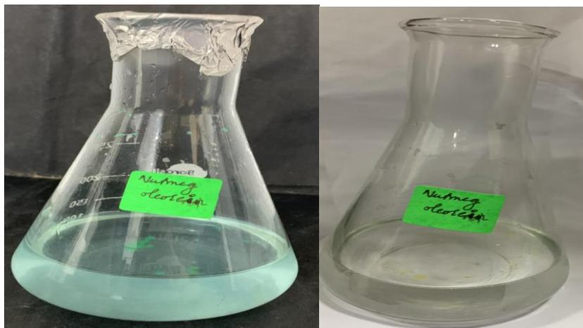
**Fig.2:** Formation of nutmeg oleoresin mediated copper nanoparticles.
