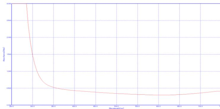
**Fig.1:** UV -Visible Spectroscopy of nutmeg oleoresin mediated copper nanoparticles .
