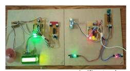
$Here, the ERV and non-ERV are displayed in working\ state\ where$ and FRV acts as a sender non-ERVactsasareceiver.Inordertoreplicatethespeedof a vehicle, DC motor. The we ultras onics ensorus ed in this project detects the automatic distantceofthenearbyvehicleandsendstheinformation to the non-ERV which is displayed ontheLCD display.
