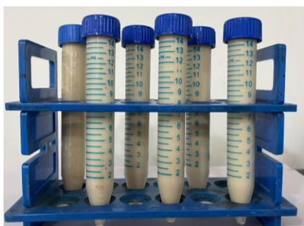
Figure 4: Tubes ready for Centrifugation with TiO 2 nanoparticle mixture.
