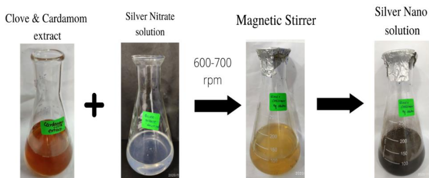
Fig.2: Preparation of Silver (Ag) nanoparticles and visual observation: 60 ml of cardamom and clove extract were added to 40 ml of Silver precursor solution and mixture was continuously stirred using magnetic stirrer at 600-700 rpm and kept overnight on an orbital shaker till color change was observed from orange-red color had transformed into a dark brown color indicating formation of Ag nanoparticles.
