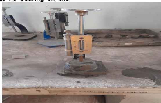
Fig 2.8: initial setting time of cement sample
