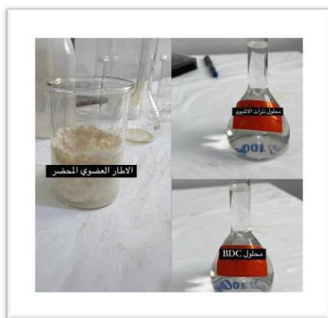
Figure (1): Prepared Solutions of Aluminum Nitrate [Al(NO_3)_3 \cdot 9H_2O] , Terephthalic Acid (BDC), and the Synthesized MOF.
