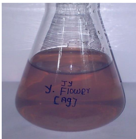
Fig 2: Formation of silver nanoparticles using Calotropis gigantea flower extract and its colour change.
