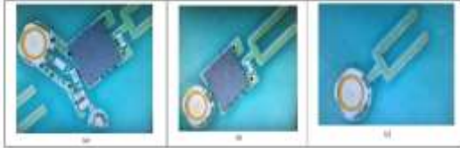
Fig 6. Fabricated element types: (a) Active antenna with the bias circuit on the same board, (b) LNA chip and inductor L1 only on the board (c) Third element type of a passive antenna for comparison
