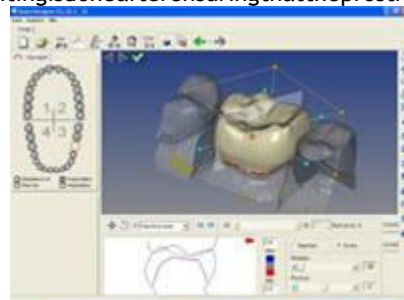
Figure 7. Display of the metal-free restoration by CAD/CAM technique. The advantages of metal-free ceramic compared to metal-ceramic works:
